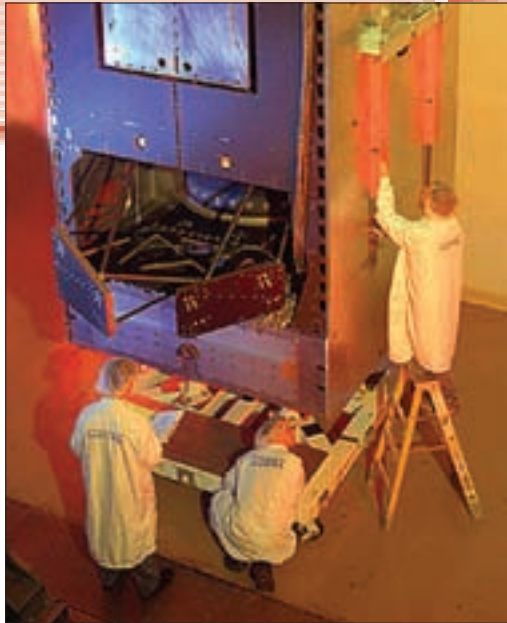
After a series of structural tests, spacecraft technicians inspect the 15-foot high panels of the iPSTAR-1 satellite. When completed, the satellite's 40-foot long solar arrays will be anchored to each of the satellite's two communication panels. Built by Space Systems/Loral of Palo Alto, Calif., the massive iPSTAR-1 satellite will be the largest commercial communications satellite ever built when it enters service in 2004.
