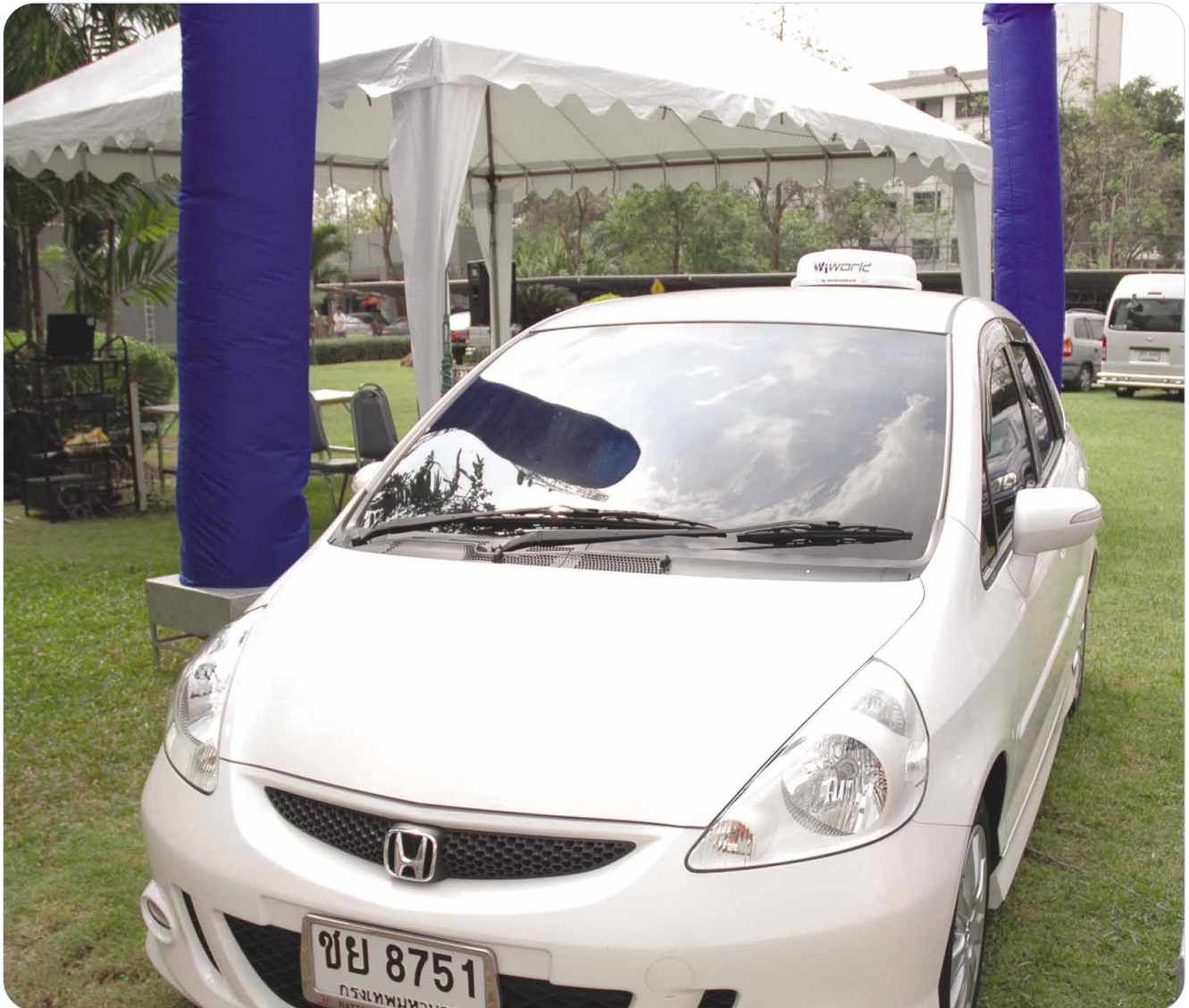
Wiworld is a mobile satellite antenna that is used to receive digital TV signals from a moving vehicle. Photo courtesy of THAI.COM.
