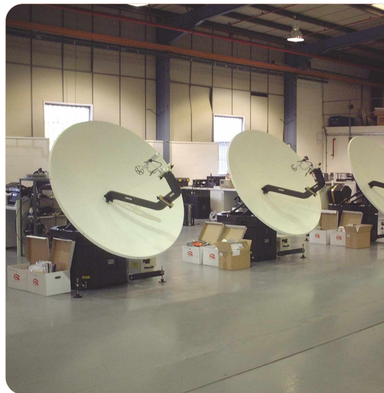
GigaSat FA-180 flyaway satellite earth stations for the BBC World Service.
