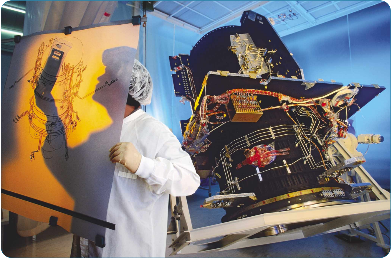
Integration of engines on a telecommunication satellite by EADS Astrium. Photo courtesy EADS / Thomas Ernsting
