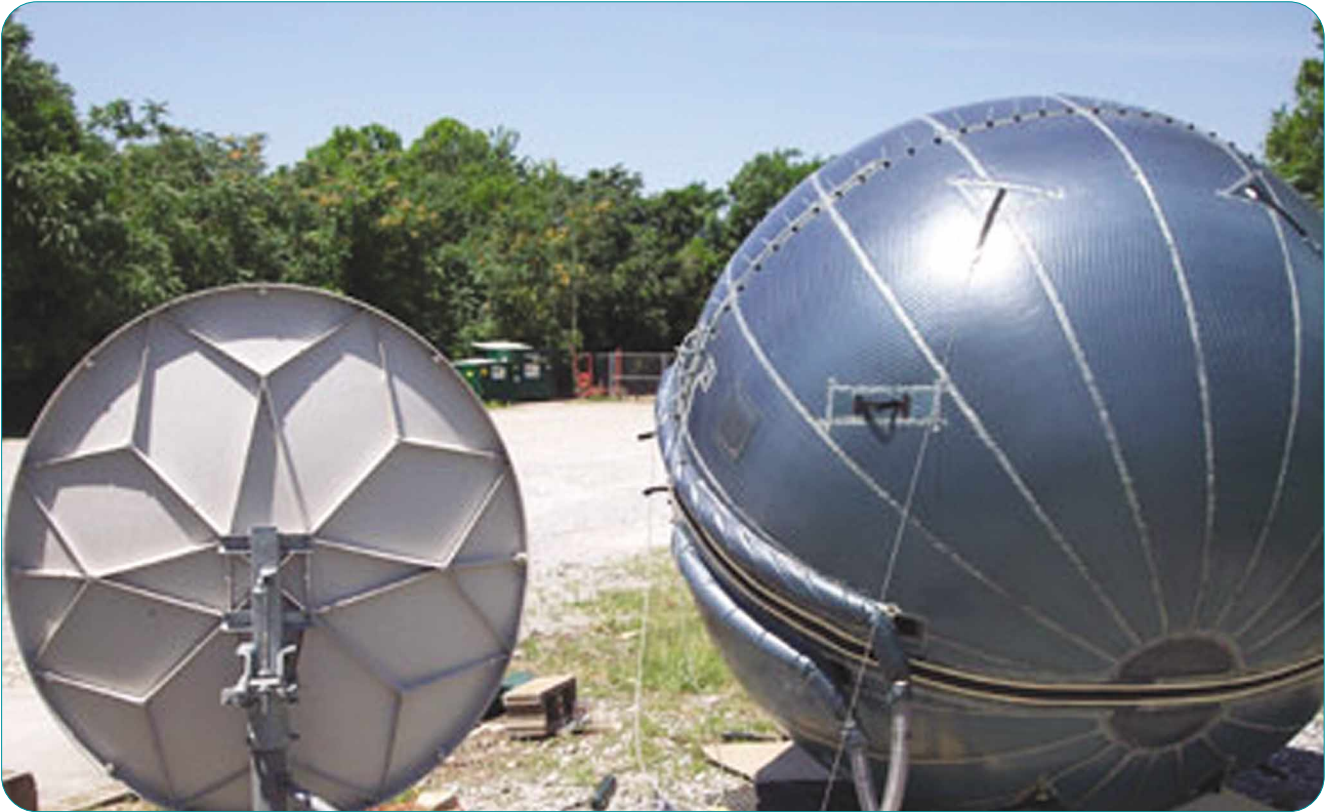
US-based company GATR Technologies provides deployable satellite solutions, including a patented inflatable antenna.
