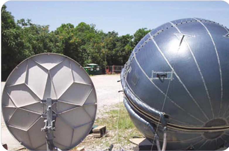
In 2006, US-based company GATR (Ground Antenna Transmit Receive) won the Product Innovation of the Year Award with their easily deployable inflatable satellite communication antenna system.
