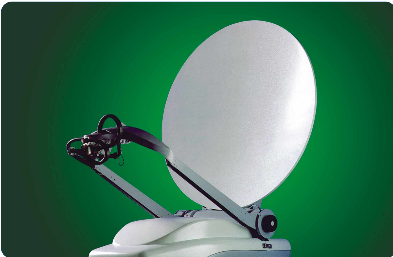
NewSwift vehicle-mounted antenna. Photo courtesy of Advent Communications.
